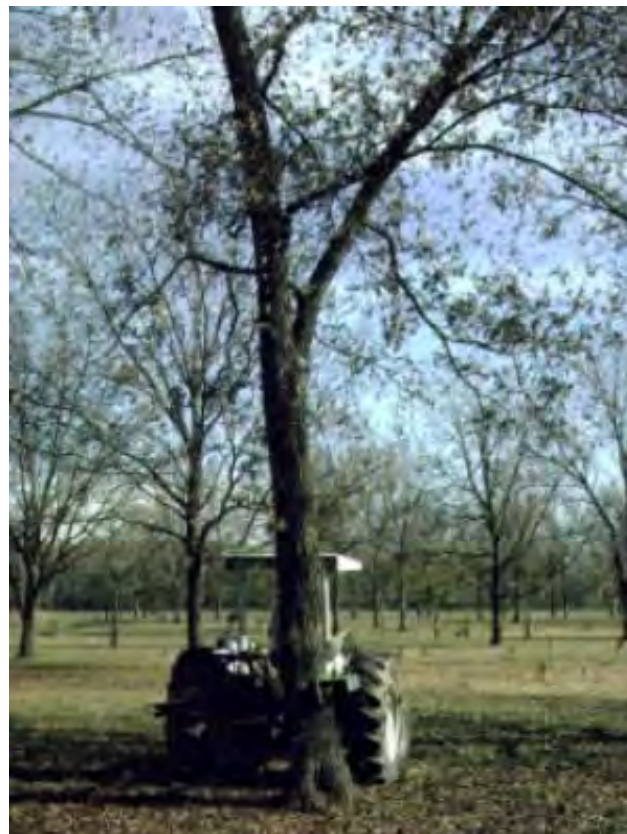
A PTO driven hydraulic pecan tree shaker facilitates the prompt harvest of the pecan crop.
