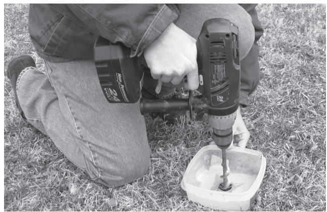
Figure 4. A power drill facilitates sampling in rocky or dry soils. Use a plastic container with a hole in the middle to collect the soil as the auger pulls it out of the ground. Empty the soil out of the plastic container into the soil sample bucket after each successful attempt to get a 6-inch core.
