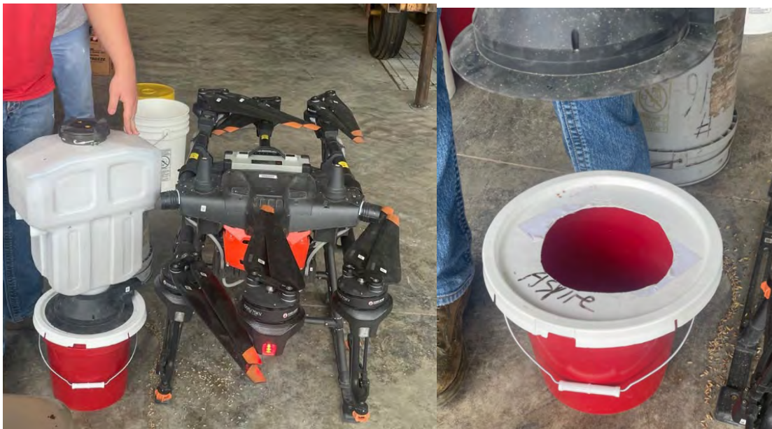
Figure 3. Spreader tank setup on a 5-gallon bucket with lid and hole cut (approximately 5-inch diameter) to collect the desired product.
