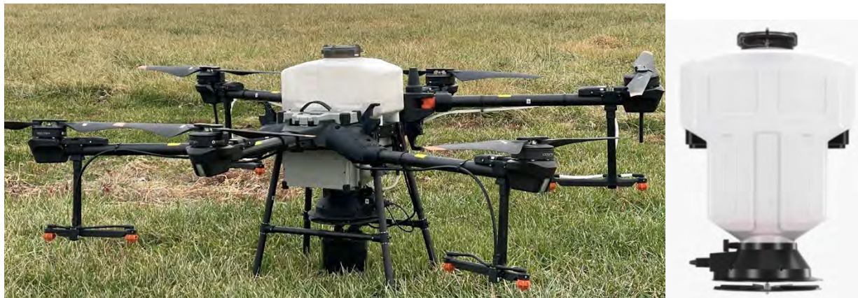
Figure 1. T-20 drone equipped with a broadcast spreader spinner disk V2.0.
